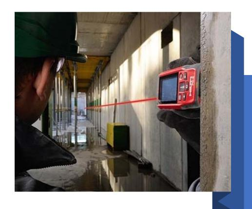
Laser distance meter: Another example of remote sensing technology
